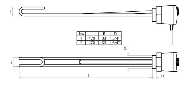
GRBT high TSE heating element is another step ELIKO has taken towards up-to-date solutions for heating technology.
